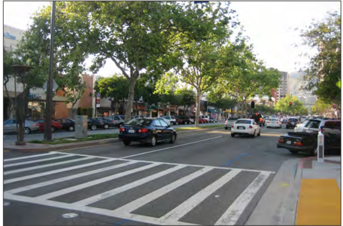
Bulbouts and a wide crosswalk provide a more inviting and safer place for pedestrians to cross the street.
