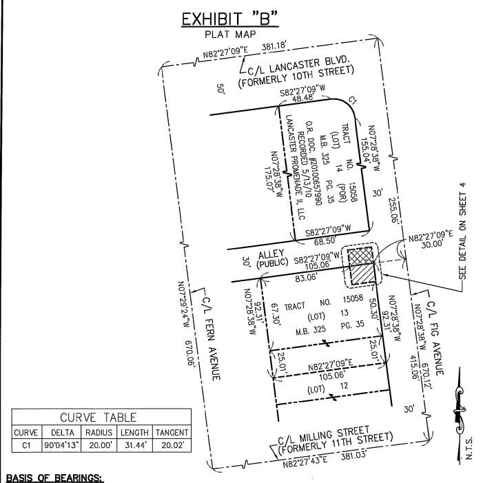
THE BEARINGS SHOWN HEREON ARE BASED ON THE BEARING OF NORTH 07'28'38" WEST BEING THE CENTERLINE OF FIG AVENUE AS SHOWN ON TRACT NO. 15058, MB 325, PG 35.
