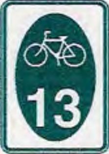
Figure 12-8: Numbered Bikeway Sign (MUTCD)
