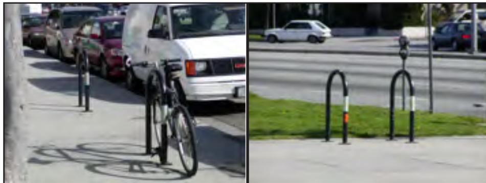
Figure 12-16: "Inverted-U" Bicycle Rack
