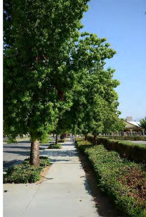
*Tree wells must meet all required clearances to ensure an unobstructed pedestrian access route*
