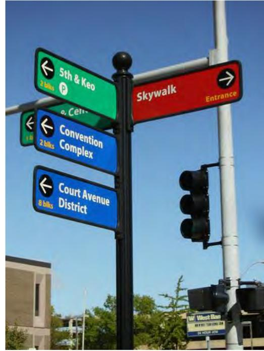
Minimize the number of sign poles by consolidating signs onto single poles
