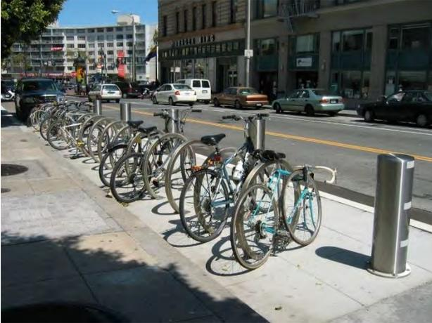
*Bicycle parking should be placed where sidewalk-area dimensions provide adequate space*
