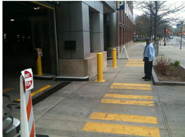
*Driveways with entry gates should ensure that the gate is appropriately placed to allow unobstructed pedestrian travel.*
