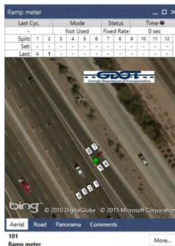
Figure 17 - Ramp meter device status view
