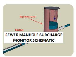
an overflow occurs. This prevents costly and messy sewer overflows. Surcharge monitors are currently installed at ten locations throughout the City which had previously experienced sewer overflows.
