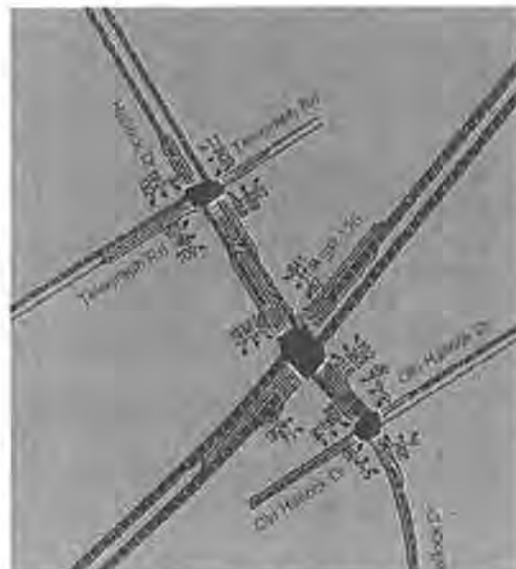
Sample Synchro Network for Operational Analysis
