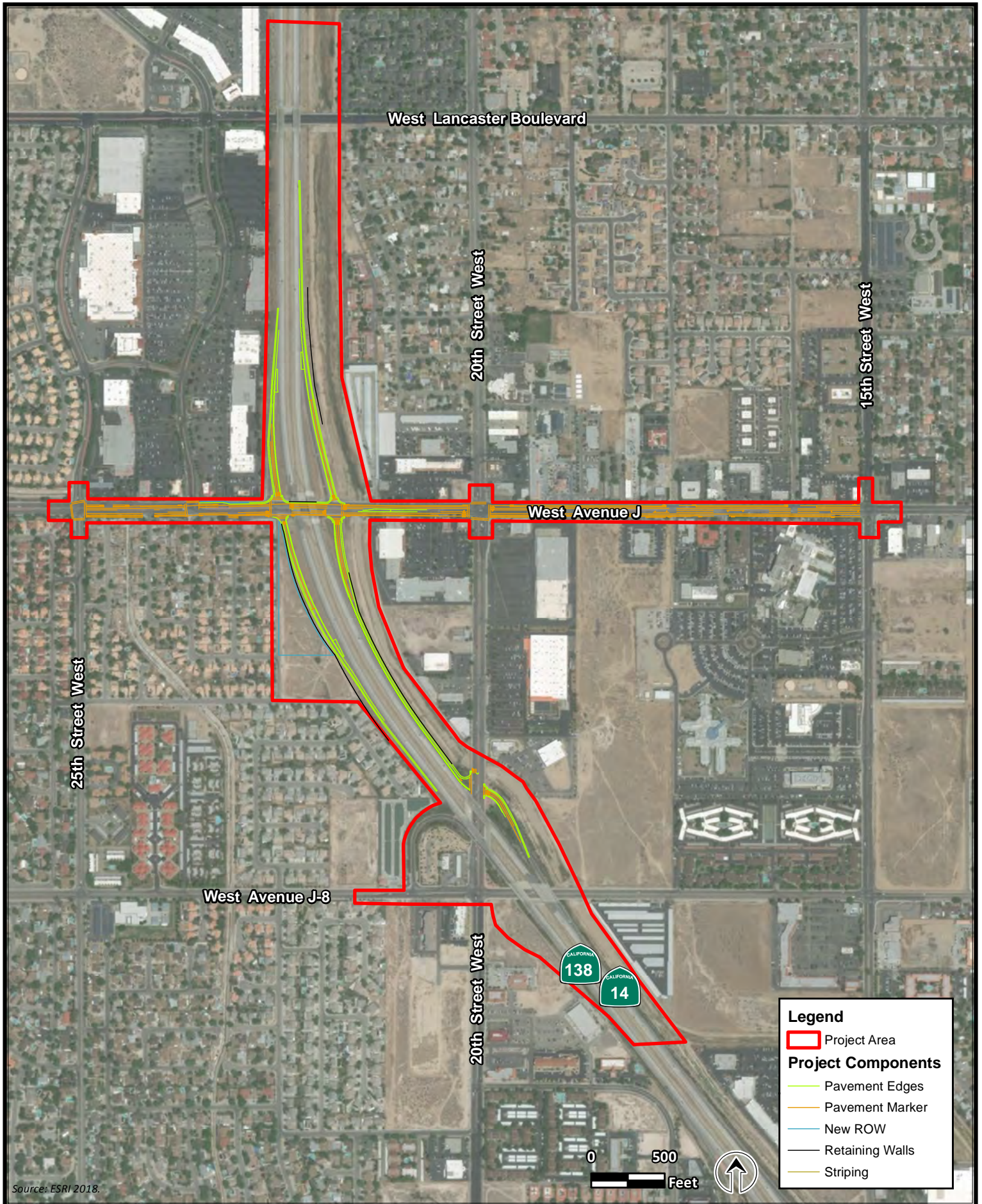
FIGURE 2-4. ALTERNATIVE 3 LAYOUT SR-14(SR-138)/Avenue J Interchange Improvements Project
