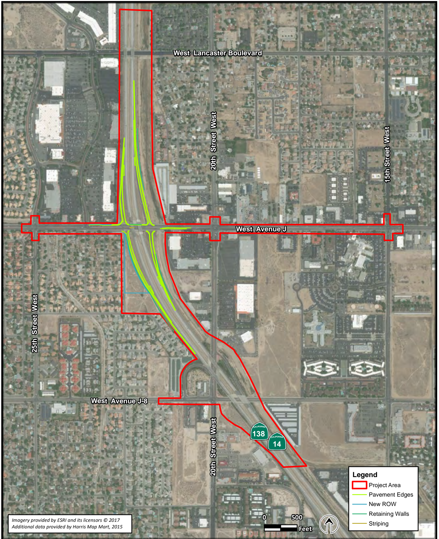
FIGURE 2-2. ALTERNATIVE 2A LAYOUT SR-14(SR-138)/Avenue J Interchange Improvements Project
