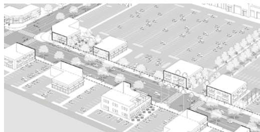
Example of Building Placement at Build-To Line for 50% of Street Frontage Diagram Courtesy of Sargent Town Planning
