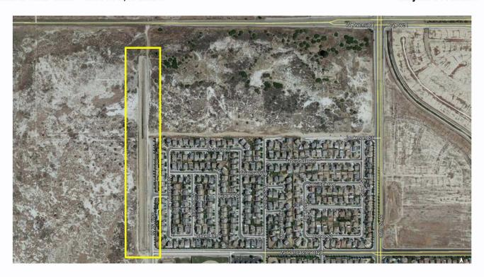
Basin needs the floor elevation reistablished to increase capacity. (Assumed average depth of removal is  $\pm 1/4$  of volume, approx. 1,800 CY; survey to be performed in-house and will contract regrading of channel.)
