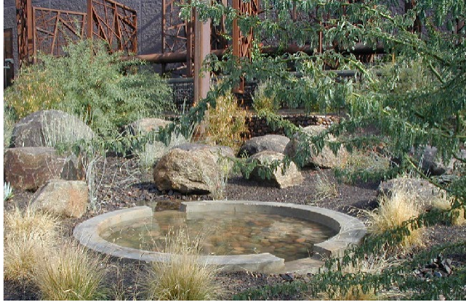
Cisterns can be used to store rainwater. They may either be above ground tanks or integrated into the landscape.
