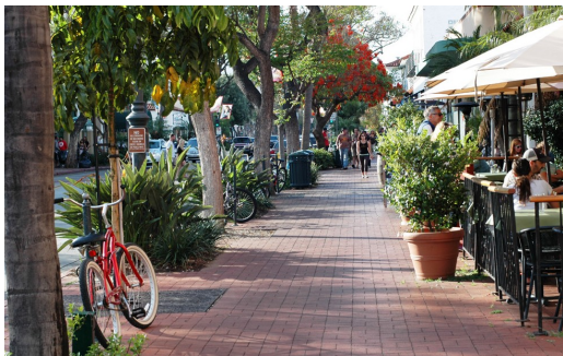
Urban frontage in a main street environment with clearly articulated curbside, landscape, pedestrian, and café zones.
