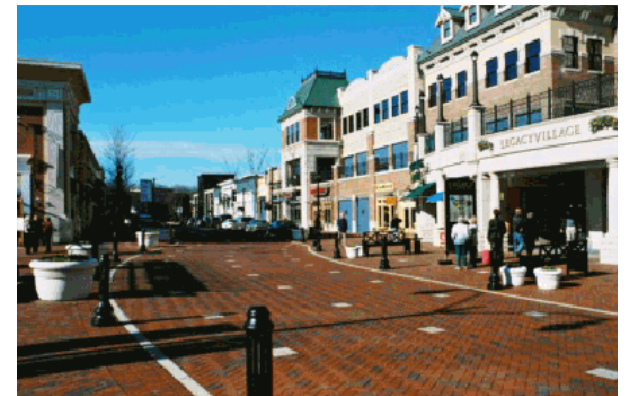
•Decorative paving, curb-less condition and bollards give priority to comfortable pedestrian access and safety
