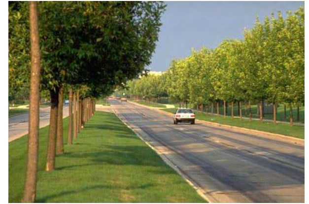
•Wide planted median and tree lawns with regular planting of canopy trees
